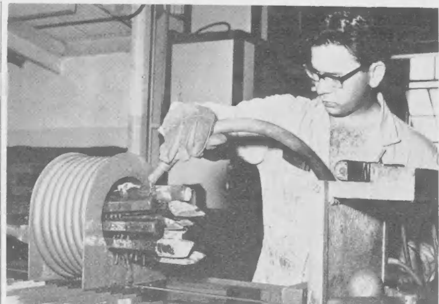
PAVEMENT BREAKERS' bits receive the magnaflux treatment directed by Alexander DeKort, a six-month trainee from HTS in Breda, Holland. Mr. DeKort will spend three months with the Equipment Inspection Group and three months in Process-Engineering.
